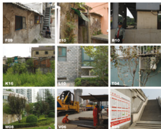
4. Grid mapping. Taking a photograph facing in the same direction at each point of a pre-defined grid allows for the survey of the qualities of a given site, and also, if done periodically, for the tracking of changes on site over time.
