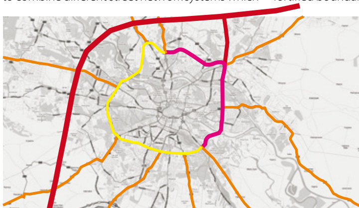
2. Prospective radial-circular routes development in Wrocław. Red - motorway bypass, orange - access roads, yellow - existing innercity ringroad, pink - planned segment of innercity ringroad.
