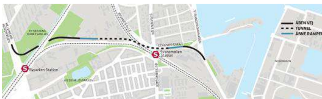
Figure 4. The Proposed New Nordhavnsvej Link in Copenhagen. Legend: Black line: surface road; black dotted line: road tunnel; blue line: surface ramps. Source: Municipality of Copenhagen (2011).
