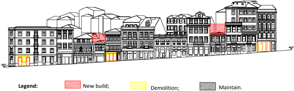
Figure 4: Elevation of proposed intervention, Mouzinho da Silveira Street. Source: Strategic Document to Ponte’s Nova Intervention Unit.
