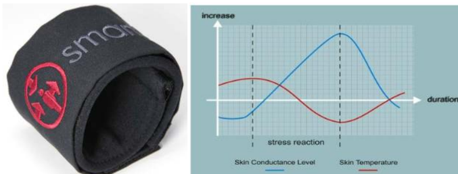
Figure 1: BMS Smartband ( www.bodymonitor.de ) & physiological patterns defining a stress reaction
