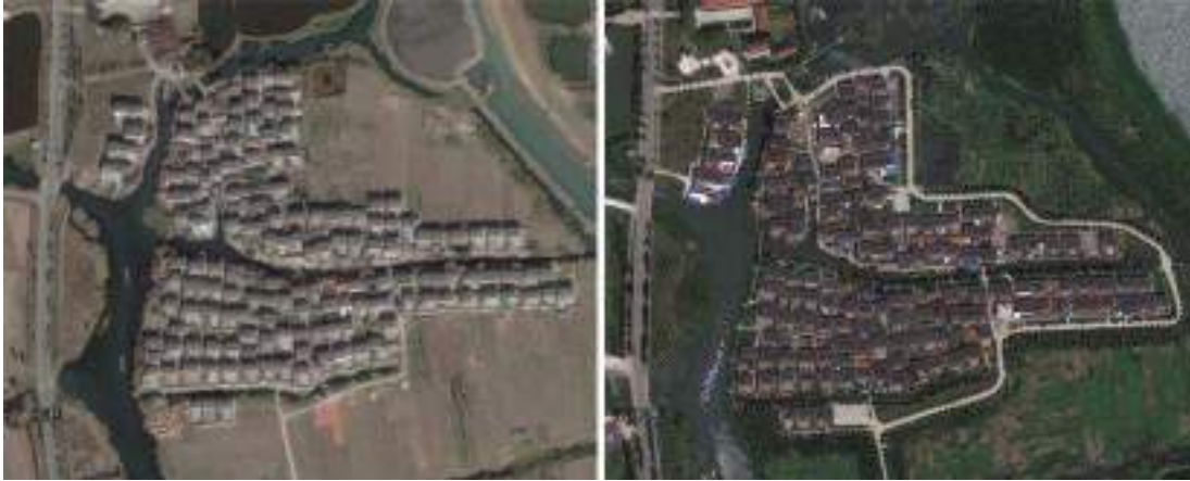
Figure 13. Aerial photos of Study Case 2, Chuodunshan Village, taken before and after the improvement of public realm. The outer service road and the footpath on the south bank of the east-west canal were added.
