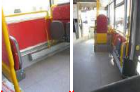
image 4. Depending on the configuration of the bus, there may be room for 2 to 5 prams. The figure on the left shows the pram area directly opposite the mid exit doors. The figure on the right is adjacent to the mid exit doors. There are some bus configurations (mainly articulated buses) that have both pram areas.
