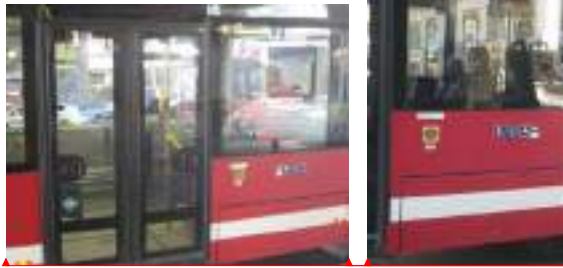
image 3. Button on the exterior of the buses by the mid exit door to allow parents with prams and people in wheelchairs to enter the bus easily.
