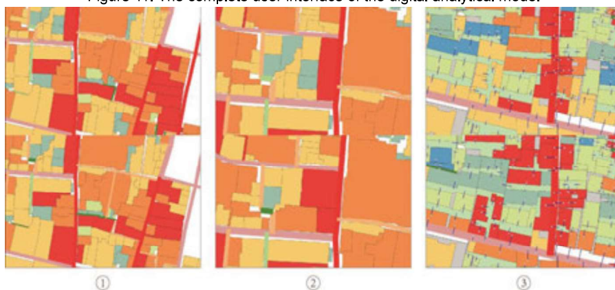
Figure 12. Users can operate data by adding or removing roads (left), redefining plots (middle), and adding or subtracting the connection lines (right) through the digital analytical model.
