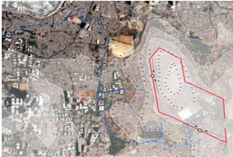
Figure 5: Satellite imagery of the site showing the boundary wall of the facility in red, overlaid with GIS based contour show direction of water flow (indicated with arrows), and natural drainage pathways in blue (Malad Wall Collapse, 2019)
