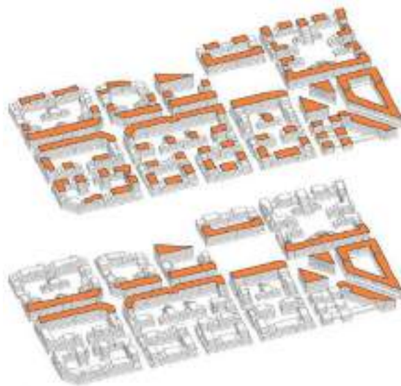
Figure 8. The analysis of the solar potential on new roofs: above, the quantification of available roofs, and below, the suitable areas to be connected in a closed network.
