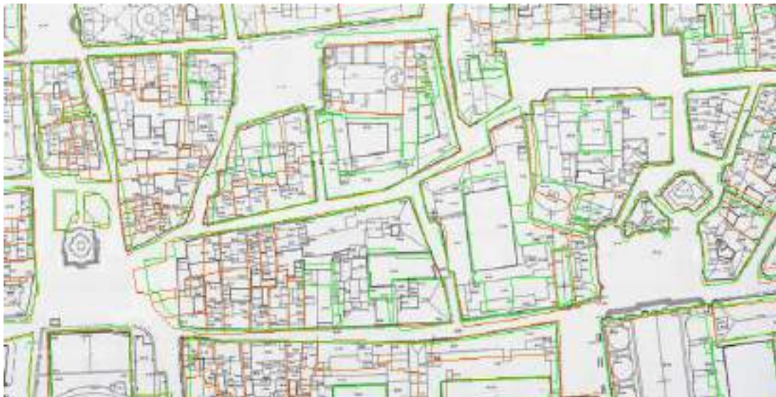
Fig. 4: The Pio-Gregorian urban cadastre of Rome (1820s) is superimposed to the Nolli plan (1748) and compared with the city plan of the area today
