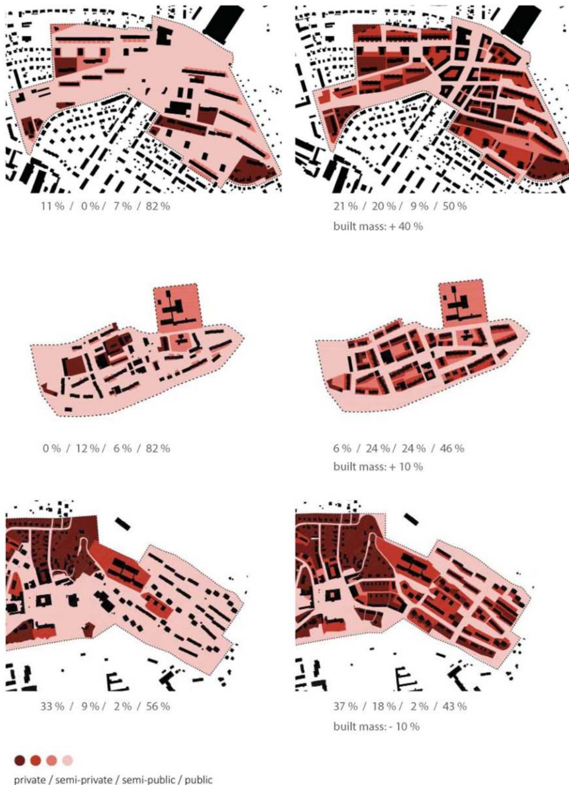
Fig. 05. Introducing broader variety of spaces with different level of privacy into housing estates fabric; top — Skalka in Prague, middle – Růžový Vrch in Karlovy Vary, bottom – Sychrov in Vsetín; left: current state, right: rearrangement proposal; source: Housing estates, what's next project case studies, Kohout–Tichý studio FA CTU in Prague, M. Decker, T. Kafková, T. Vrbová
