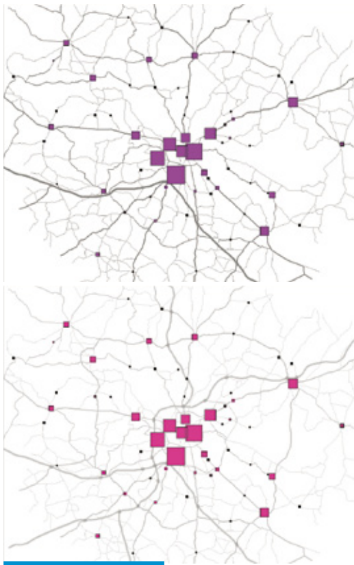
9. Application of the model to examine the impact of different networks on the Metropolitan Area of Wrocław: results after 100 iterations of modelling conducted respectively on the real and the planned network from initial real origins and an even distribution of destinations; selectivity equals 0,000250, 0,000050 and 0,000005 ('sharp')
